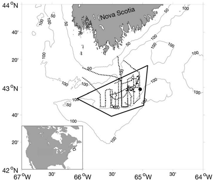
*Figure 1.* Bathymetric chart showing the 2014 visual survey track-lines (dotted) in the Roseway Basin Area To Be Avoided (ATBA; polygon) and locations of bottom mounted PAM systems (solid circle). Similar figures for each survey day of each year are provided in Fig. S1A–E.
