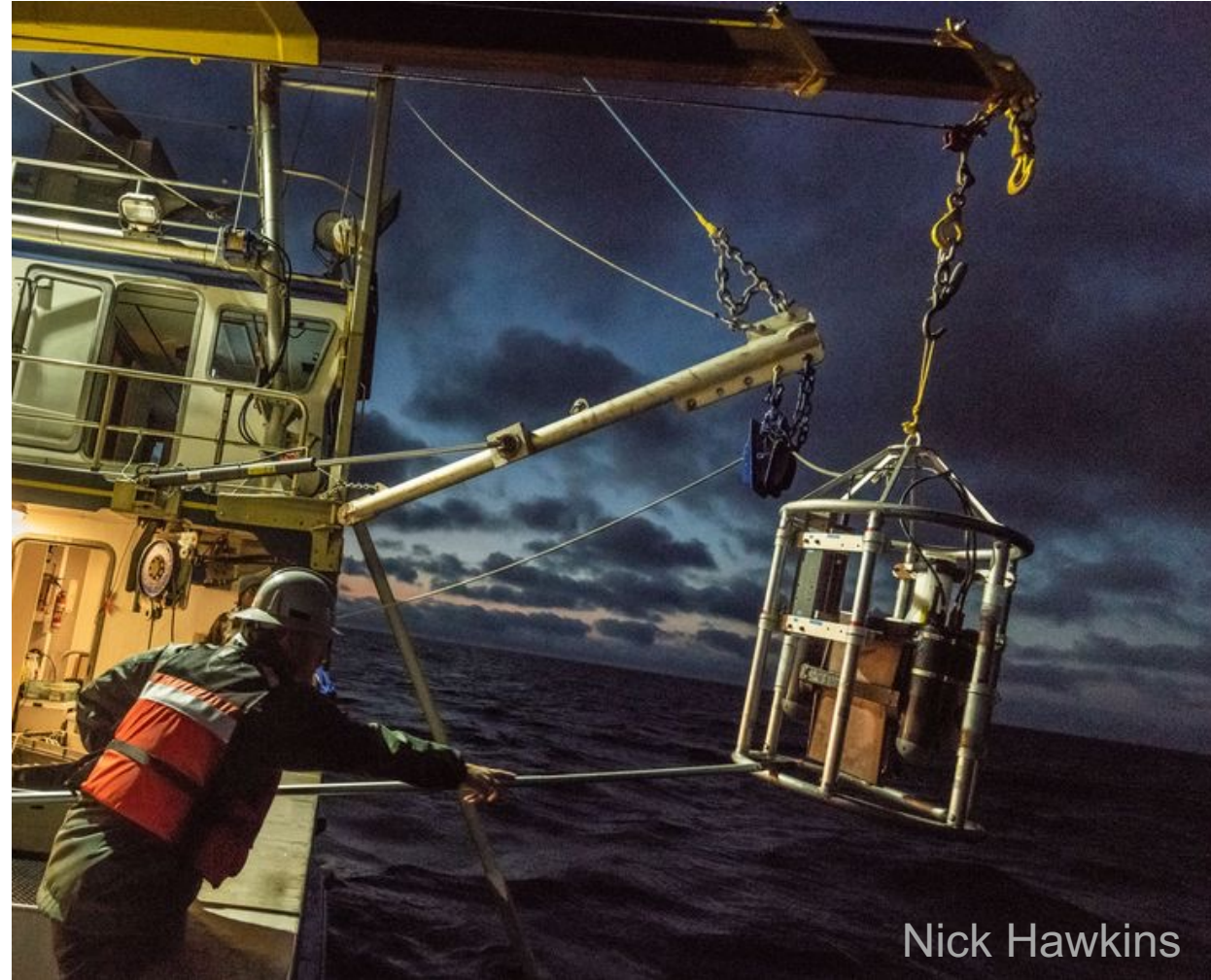
Profiling Cage: CTD + Optical Plankton Counter (OPC)
